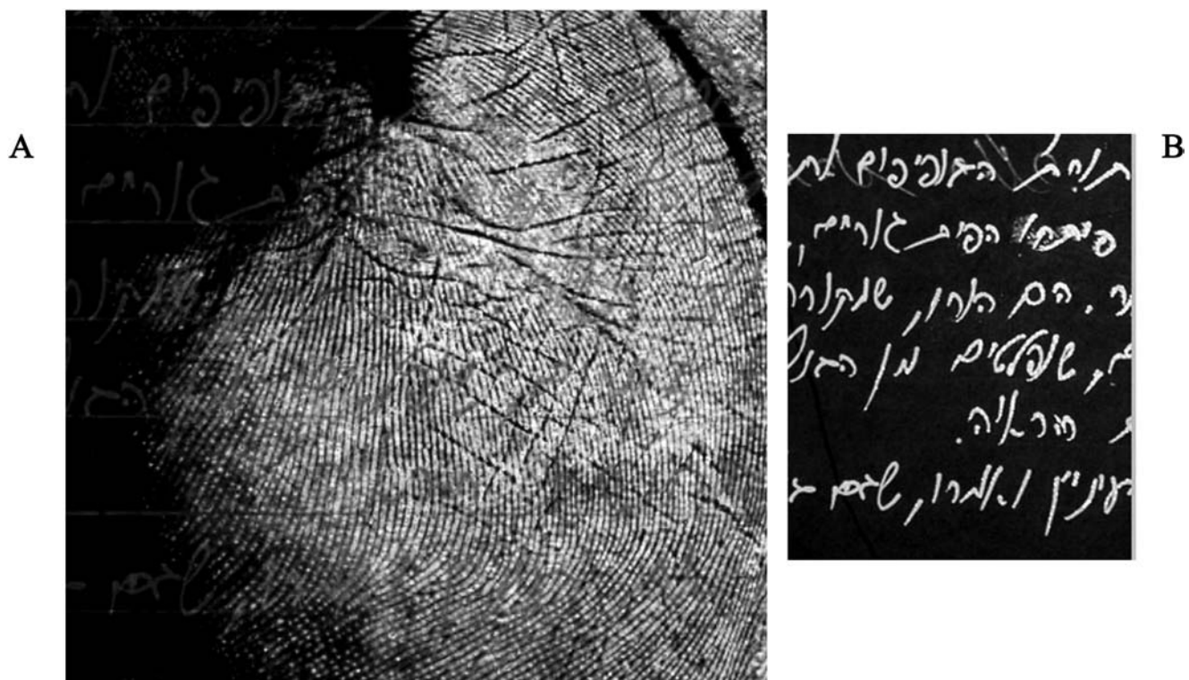
FIG. 3—(A) palm print developed with genipin on a document written with ink containing fluorescent ingredients and recorded under fluorescence conditions (excitation at 590 nm, cut-off Kodak red filter No. 92); (B) same document observed at 505–530 nm (DFO conditions).
